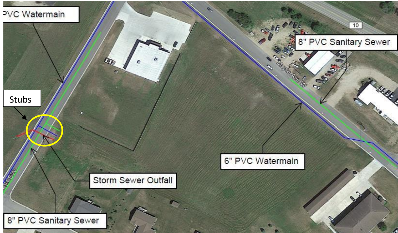
Figure 3: Utility access for both water and sewer
